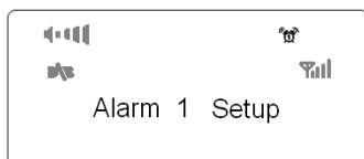
2. Press **SELECT** to confirm '**Alarm 1 Setup**', you will enter the '**Alarm 1 Wizard**', follow the instructions on the display to configure the following parameters:
