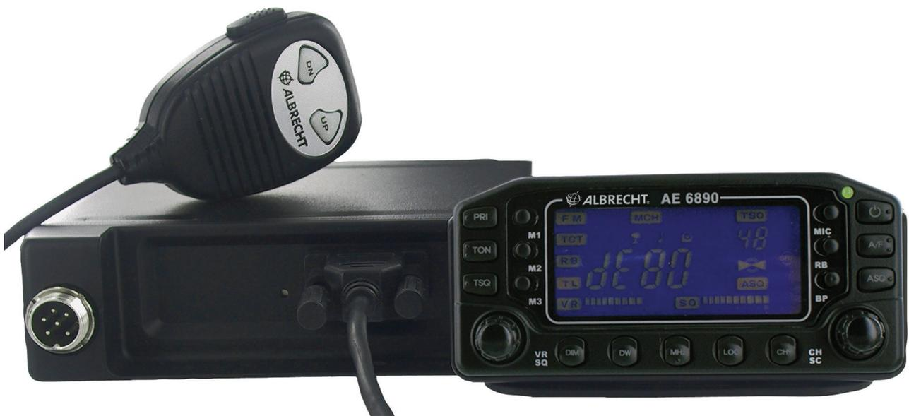
The front section can be removed after opening 2 fixing screws on the bottom side.
