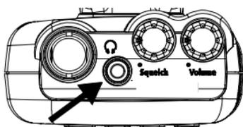
For private listening, you can plug a 3.5 mm mini plug earphone or mono or stereo headphones (not supplied) into the headphone jack on top of your scanner. This automatically disconnects the internal speaker.
