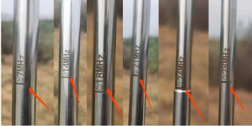
• Although there are reference points, you might still need to do fine adjustments to the length of the whip antenna until you get a sensible VSWR readings(From an in/external VSWR meter, VNA or antenna analyzer).
