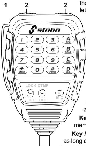
**Key F/C [A]** Switches the display over to indicate either the frequency or the channel (as F/C key on the radio set).
